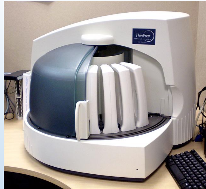
ThinPrep Imager used to image ThinPrep slides
