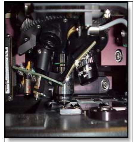
Imaging a SurePath slide in the FocalPoint Profiler
